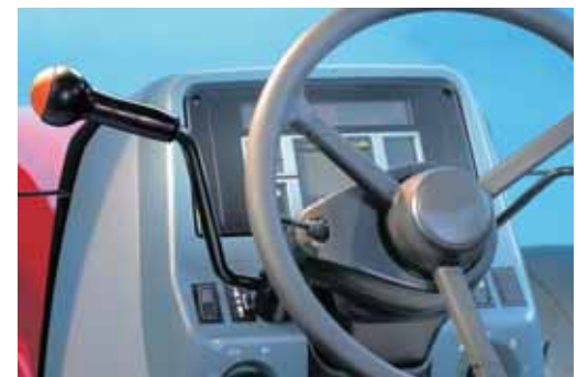
Synchromesh shuttle transmission with creep speed option for outstanding performance in the field.
